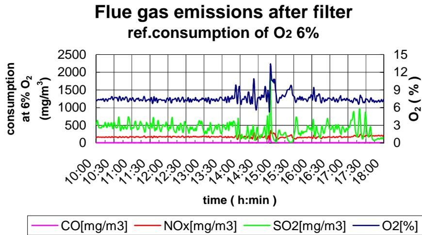
**Fig. 9** Flue gas concentration during combined combustion tests -coal 80% and 20% biofuel.
