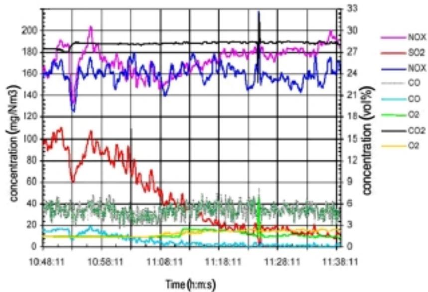
**Fig. 5** Concentration of gaseous emissions during combined combustion of coal and wood pellets in pilot fluidized bed boiler 300 kW TU Dresden. The  $\text{CO}$ ,  $\text{O}_2$ , and  $\text{NO}_x$  concentrations were each measured with two different instrument.
