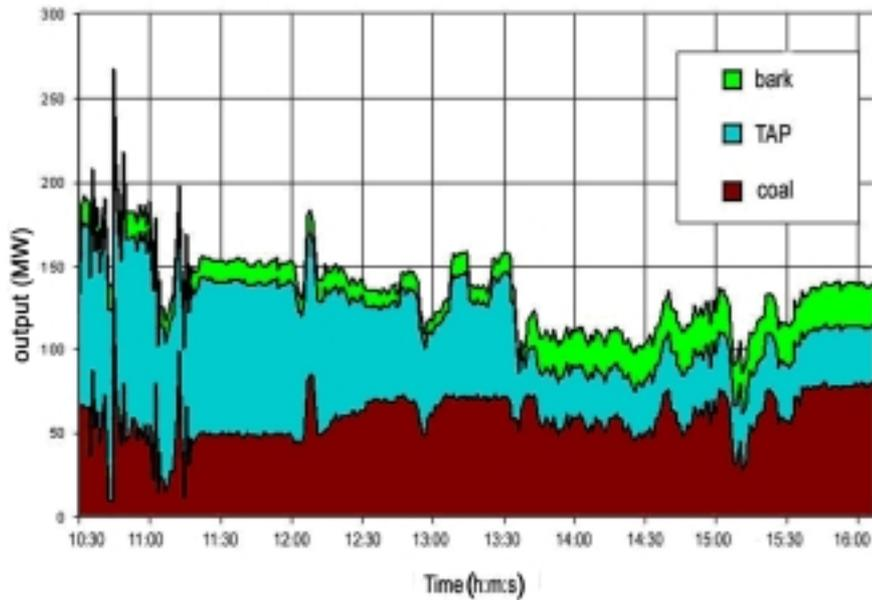
**Fig. 6** Output of the circulating fluidized bed boiler Foster Wheeler and distribution of coal, solid alternative fuel (TAP) and bark during combustion experiment.
