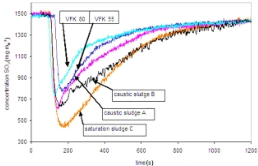
Fig. 12 Time behavior of concentration of  $\text{SO}_2$  on the outlet from boiler model with circulating fluidized layer after dosing the sorbent.
