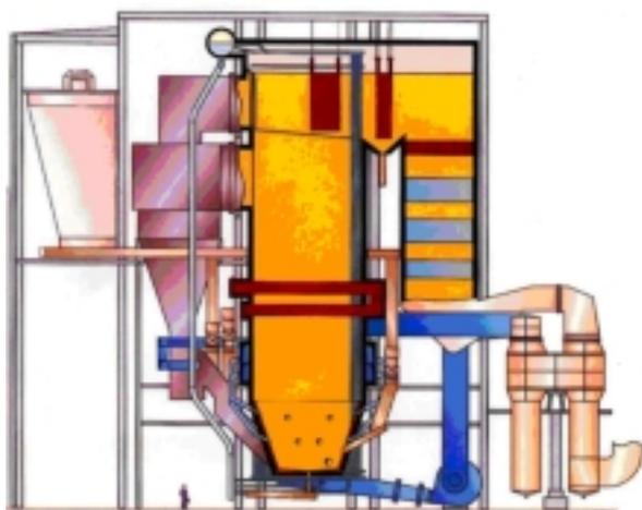
**Fig. 7** The fluidized-bed boiler Foster Wheeler 220 t/h.
