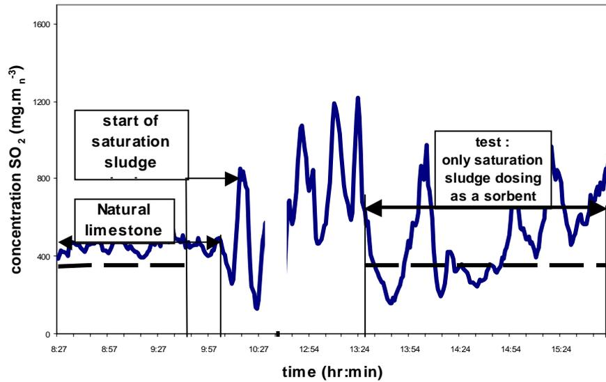
Fig. 11 Saturation of sludge dosing as a sorbent in the large FCB boiler.
