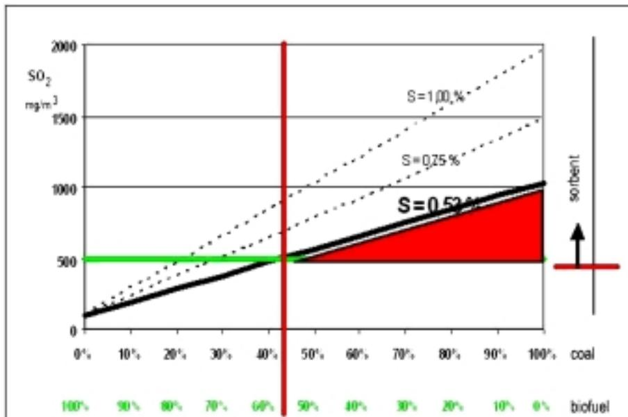
**Fig. 10** Influence of the ratio coal/biofuel on the concentration of the SO<sub>2</sub> and environmental limit.
